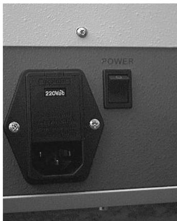
The change of the power to 110 V is demonstrated by III. After opening the cover the corresponding voltage may be set by turning it. At the same time the power fuse is accessible and has to be exchanged. The cover then has to be closed again.
